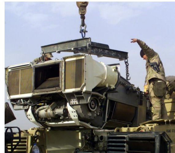
An AGT1500 Turboshaft engine being installed into a tank. The AGT1500 is the predecessor to the LV100.
