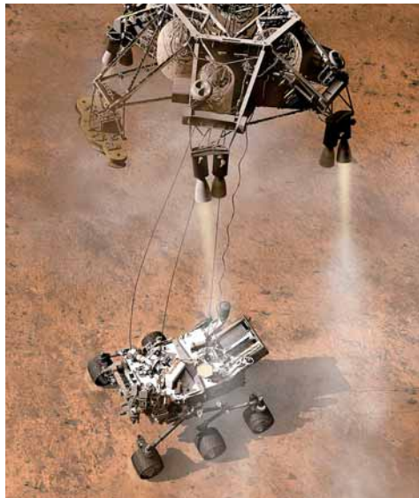
Seven Minutes of Terror. Lowering the rover to the Martian surface on cables was a particularly delicate maneuver. The landing phase was simulated 8,000 times.
