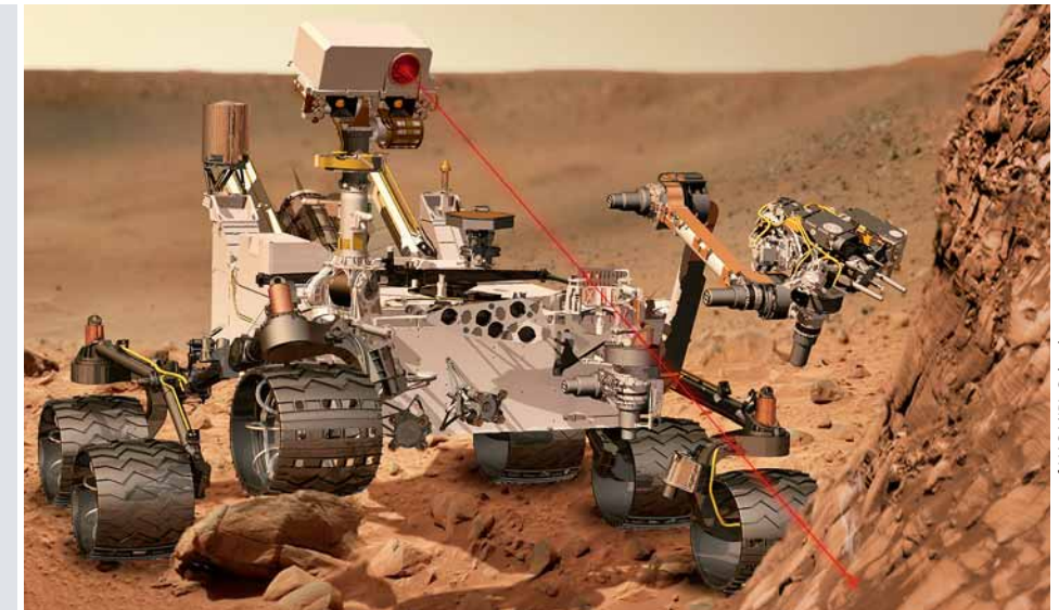
The entire unit consisted of around 90,000 parts, many of which were allowed to deviate from design by only 100 micrometers — about the width of a human hair.
