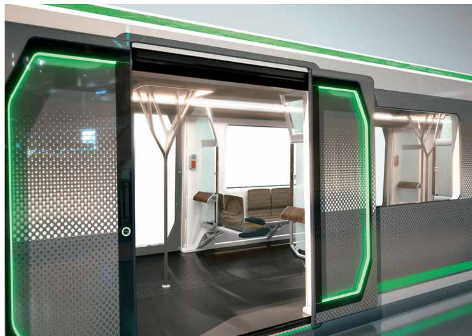
Left: Strips of colored LEDs mounted in doors fall like sand through an hourglass, indicating that the train is about to leave. Below: A simulation of passenger flow on a platform and in a railcar helped to determine the optimal door width.
