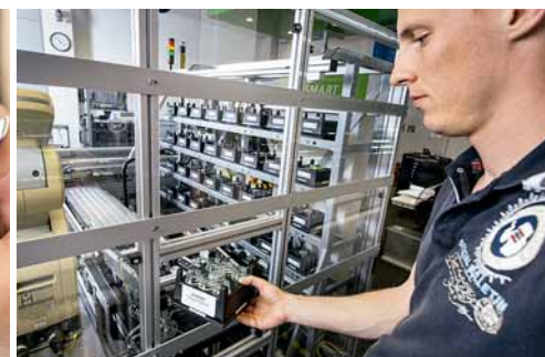
During production, merchandise is constantly scanned, producing a real-time overview. All data flows into a central collection point for processing.
