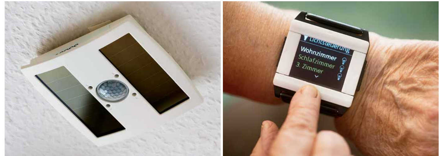
A combined movement and brightness sensor (left) and a WLAN-equipped wristwatch can trigger an alarm if something goes wrong.
