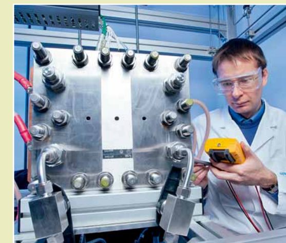
Testing a PEM-equipped electrolyzer at Siemens.
