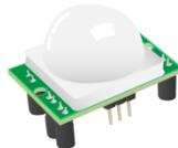
Figure 2 : Passive Infra Red Sensor
