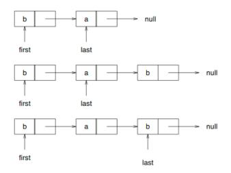
$\ldots$  unless the queue is empty, then  $\mathtt{first}$  and  $\mathtt{last}$  must both reference a new link  $\ldots$
