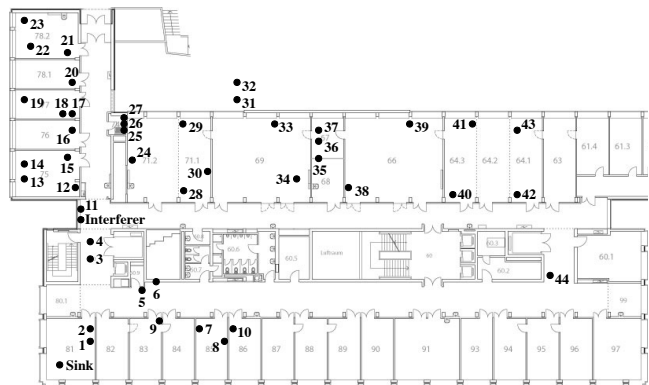
Figure 5: Testbed layout. Nodes 31 and 32 are located outside on the rooftop; the interferer is only used in Sec. 6.6.
