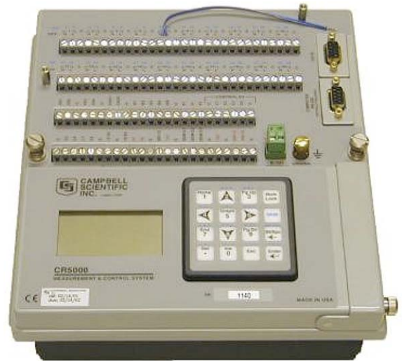
Fig. 2. A CR5000 datalogger from Campbell Scientific used for monitoring up to 40 sensors. Data is either manually retrieved from its onboard storage or transmitted to a central receiver [4].
